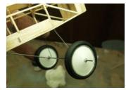
If you want to make the wheels very tough shoot about 1 to 3cc's of polyurethane glue inside the wheel and about 5 drops of water. Install t
