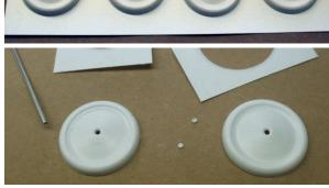
on the axle tube and rotate to check for true turning. Rotate one half of the wheel and check again. When the best match has been made mark the wheel. Apply model cement to the edges of the wheel and bond the halves and allow it to set completely.
