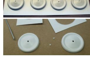
on the axle tube and rotate to check for true turning. Rotate one half of the wheel and check again. When the best match has been made mark the wheel. Apply model cement to the edges of the wheel and bond the halves and allow it to set completely.
